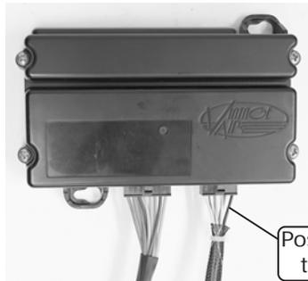
**NOTE: ECU must be placed away from water and humidity, and also be accessible for servicing. If relocating, connectors must be positioned towards the bottom.**
