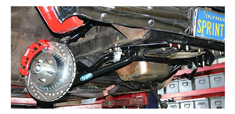
PLEASE NOTE: The installer needs to make sure that nothing can make contact with a brake hose, caliper, or other brake component at any point through the entire range of steering and suspension movement. The installer also needs make sure none of the steering or braking components can become bound or jammed at any time through the range of suspension or steering movement.
