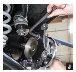
10.Install the hub to the spindle and tighten all three bolts, recommended torque spec is 96 foot lbs. (Photo J)
