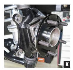
11. Next, if you intend to set up the spindle and hub for OE wheel offset. install the rotor spacer to the outer face of the hub. (Photo K)
