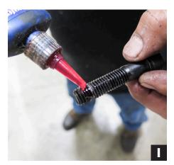
9. Apply thread locker to the hub bolts before installation. (Photo I)
