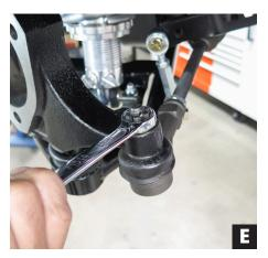
4. Attach the tie rod end to the steering arm of the spindle and tighten castle nut. (Photo E)
