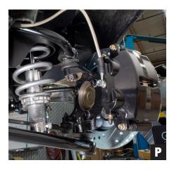
16. Proceed to finish the installation of your chosen Corvette big brake kit on your Mustang II Corvette-Style Spindle & Hub Assembly. (Photo P)
