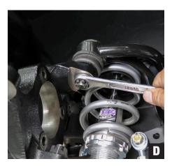
3. Then bring the upper control arm down and install the ball joint stud into the top of the spindle. Tighten both upper and lower castle nuts. (Photo D)
