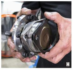
8. Next, if you are setting up the spindles and hubs for either negative 1/4" or OE offset, install the hub spacer on the back of the hub assembly. (Photo H)
