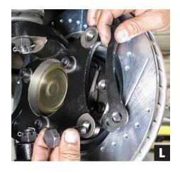
12.To install the brake caliper to the spindle, first install the rotor and thread on two lug nuts to hold the rotor flush against the hub. Both caliper spacers will be used to mount the brake caliper. (Photo L)
