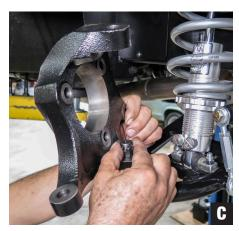
2. Begin by installing the spindle on the ball joint stud of the lower control arm (Photo C).
