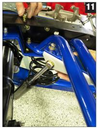
Carefully raise the rear end to locate and install shock into the new upper bracket. (Fig 11)
