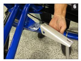
Install the upper Shock Relocator bracket with the slotted hole forward; the shock will mount at the rear side of the bracket. (Fig 6)
