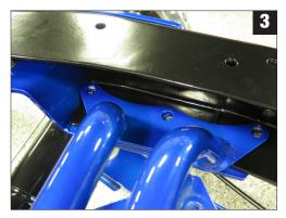
Locate the series of factory rivets attaching the crossmember to the frame—there are 3 on the upper framerail flange and 2 on the lower flange. There are various methods in which to remove heavy sheetmetal rivets; grinding the head flush on one side and drilling out (with the additional aid of a hammer and punch) usually works well. (Fig 3)
