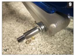
CPP offers new lower shock studs (CPP-SMS) as well as three shock options: (CPP-4163G) stock; (CPP-4095G) 2-4" lowered; and (CPP-4052G) 5" lowered. (Fig 9)
