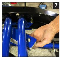
Note: bolts (at least the rear one) must be inserted from the bottom so as to not interfere with the shock absorber itself. (Fig 7)
