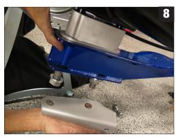
The lower shock brackets mount (in the stock location) with the stud hole facing in towards the driveshaft, in the forward position. (Fig 8)
