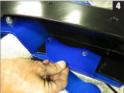
The CPP tubular rear shock crossmember will locate directly off the existing lower two holes as well as integrate the upper mount for the coil spring. The two-hole shims are for use on frames that have the additional gussets-they go between the crossmember and the lower framerail flange. (Fig 4)
