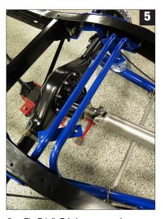
The Totally Tubular crossmember mounts with the shock perch flanges pointing inwards, toward the cab. (Fig 5)
