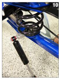
With the shock attached to the lower mount, reinstall the coil spring; the upper pocket will use the supplied hardware to attach and secure the shock crossmember. (Fig 10)
